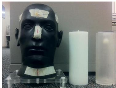
**Figure 2.** Head phantom with dosimetry insert (L) and imaging insert (R)
